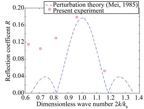
Fig. 9. Comparison of the Bragg resonance reflection coefficient between the present experiment without a point absorber at the water depth of 0.8 m and perturbation theory (Mei, 1985).
