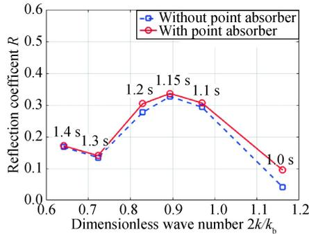
Fig. 6. Reflection coefficient of the Bragg resonance by wavy bottoms with and without a point absorber at the water depth of 0.7 m.
