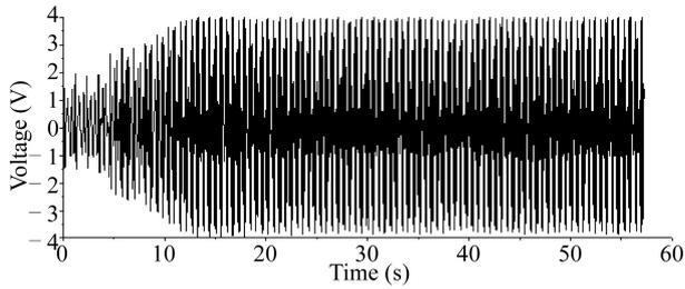
**Fig. 10.** Time series of the voltage extracted by a linear generator before and after the Bragg resonance occurs ( $T=1.15$  s,  $h=0.6$  m).
