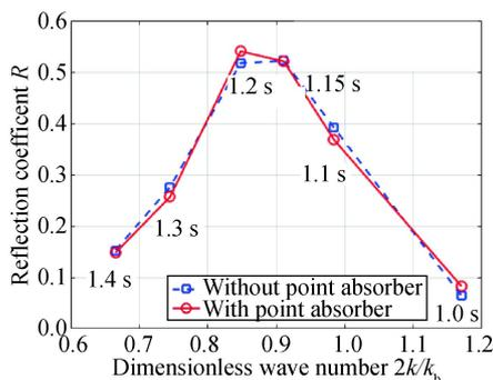
**Fig. 4.** Reflection coefficient of the Bragg resonance by wavy bottoms with and without a point absorber at the water depth of 0.6 m.
