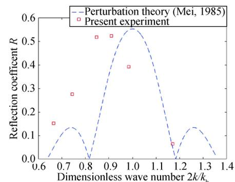
**Fig. 5.** Comparison of the Bragg resonance reflection coefficient between the present experiment without a point absorber at the water depth of 0.6 m and perturbation theory ([Mei, 1985](#)).
