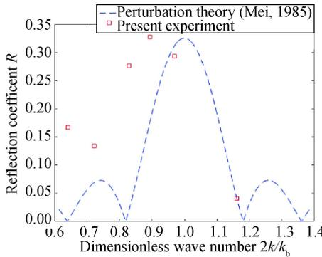
Fig. 7. Comparison of the Bragg resonance reflection coefficient between the present experiment without a point absorber at the water depth of 0.7 m and perturbation theory (Mei, 1985).
