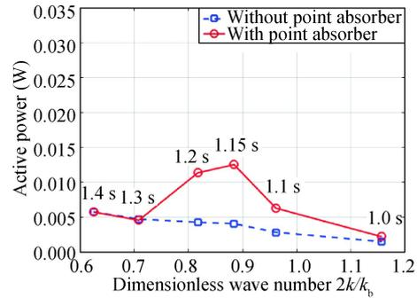
**Fig. 14.** Comparison of the active power extracted with and without Bragg resonance ( $h=0.8$  m).
