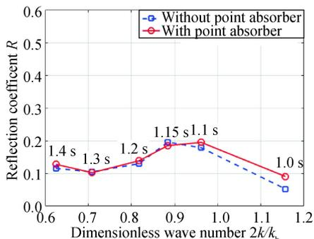
Fig. 8. Reflection coefficient of the Bragg resonance by wavy bottoms with and without a point absorber at the water depth of 0.8 m.
