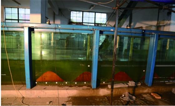
**Fig. 2.** Continuous sinusoidal periodic topography on the bottom of the flume.
