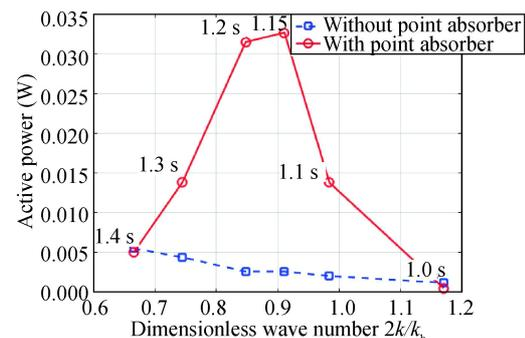
**Fig. 12.** Comparison of the active power extracted with and without Bragg resonance ( $h=0.6$  m).
