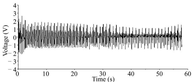
**Fig. 11.** Time series of the voltage extracted by a linear generator on the flume of a flat bottom (with the same incident wave in Fig. 7).
