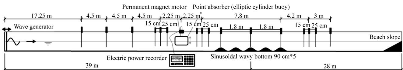
**Fig. 1.** Experimental set-up of the wave-power enhancement by Bragg resonance.
