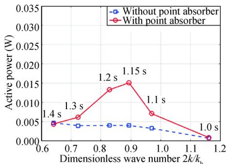
**Fig. 13.** Comparison of the active power extracted with and without Bragg resonance ( $h=0.7$  m).
